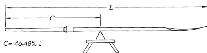
Figure 3. Centre of Gravity of The Oar
