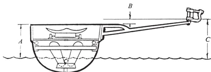
Figure 1. Immersed Hull Measurements
